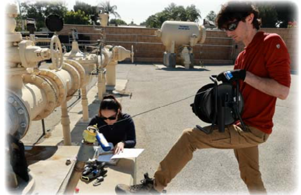
WM Staff Measuring Groundwater Level at CDA Well Site
